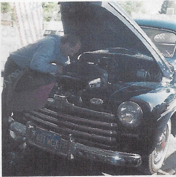
All hoses off. Air and water power flush the block from the top.
